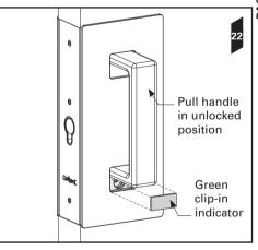
**23**. If installing a handle with snib both sides, fit the clip-in indicators to both sides.
