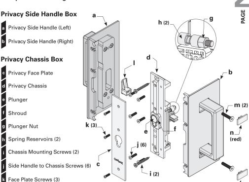
n Note: Components will vary between the 'Snib/Emerg', (green) 'Snih/Snib' and 'Snib One Side' versions. Straight handle option shown.
