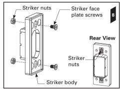
**9**. Insert the striker body, with the striker face plate screws and the striker nuts attached, into the cut out in the closing jamb.
